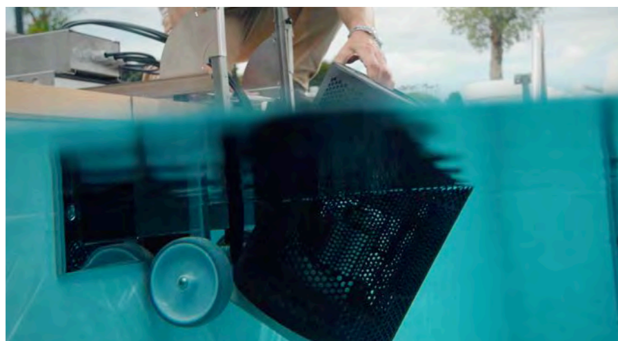
2. Unclip the rotating bracket (with EVastream) on both sides and place it upright. Lower the EVastream Move into the water.
