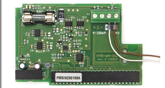
Insert the two white and brown wires into the connection terminals of the PM5-mA-IN2 plug-in module and fix them with a small screwdriver. Check, if the cables are properly fixed. Take care of the white and brown colour code label below the terminal:
