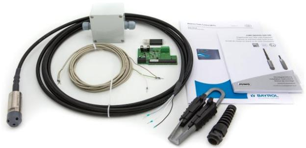
The Balance Tank Control is an add-on to the BAYROL PoolManager®, PoolManager® PRO and Analyt controllers. It measures the water level in the balance tank in centimetres. A very robust hydrostatic sensor (pressure sensor) made of titanium is used for the measurement. The sensor provides a 4-20 mA signal.
