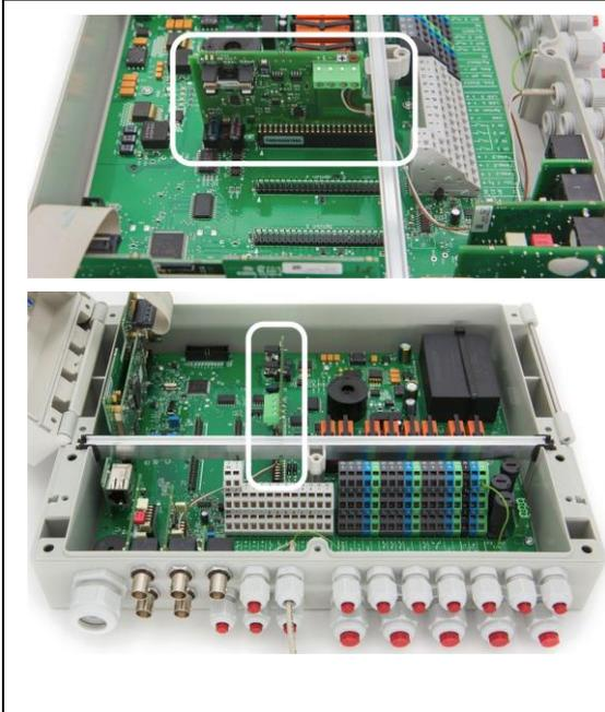
These pictures show the correct position of the PM5-mA-IN2 plug-in module and the cables after installation.
