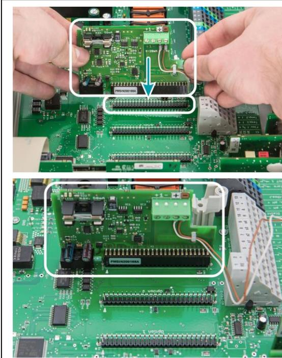
Move the PM5-mA-IN2 plug-in module to the correct position and insert it carefully into the plug-in connector 3 (on the right).
