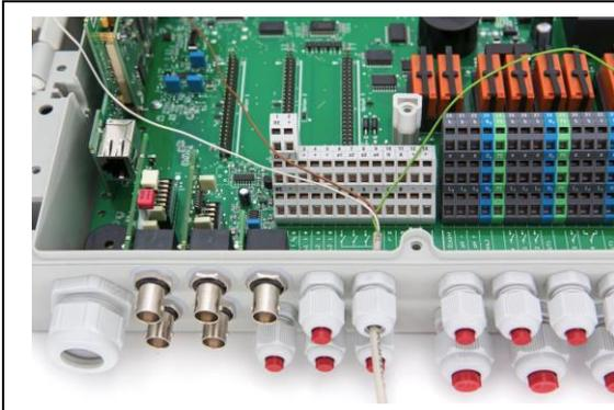
Remove the cap from one of the smaller cable glands in the upper row of your PoolManager®, PoolManager® PRO or Analyt controller and lead the connection cable through the cable gland.
