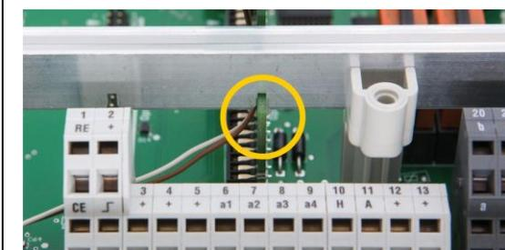
Now insert the aluminium rail at its original position. Take care that the PM5-mA-IN2 plug-in module is exactly located in the corresponding slot of the aluminium rail as shown on the picture.
