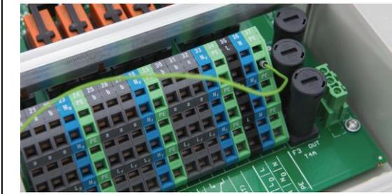
Connect the green PE (protective earth) wire to one of the green PE terminals of the controller. You can use any of the green PE terminals.
