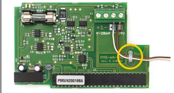
Use a cable tie (cable binder) to fix the wires firmly on the PCB (printed circuit board) of the PM5-mA-IN2 plug-in module. The cable tie is important for strain relief. You need to fasten it very firmly in order to fix the thin wires.
